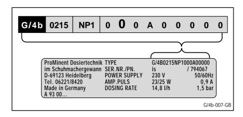
Each gamma/4 metering pump is provided with an identification plate. This can be found on the base of the pump.
