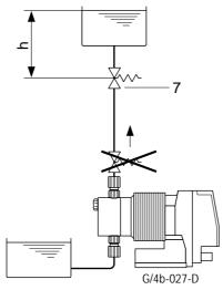
Calculation of the max. permissible line height  $\boldsymbol{h}_{\max}$  above the back-pressure valve:
