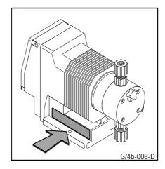
In addition to the technical basic data the IDENTITY CODE and the serial no. are specified. Both numbers are to be stated during any enquiry or when ordering spare parts as they permit a clear identification of the pump type and material variant.
