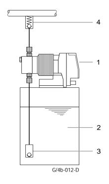
2a) Atmospheric discharge and low head
