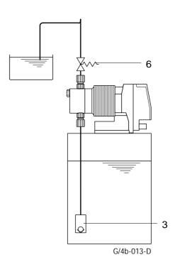
2b) Atmospheric discharge and large head
