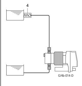
3a) With back pressure on the suction side and **large** discharge head
